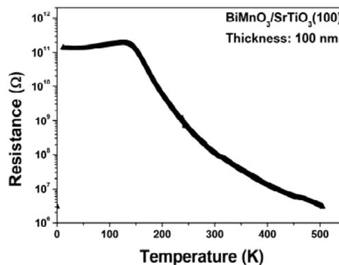
**Figure 2.** Resistance ( $R$ ) in zero applied magnetic field as a function of temperature for a BMO thin film grown onto STO (100) substrate. Below 150 K, the resistance increases very sharply. Around  $T = 135$  K, we can see the onset of ferromagnetic order.
