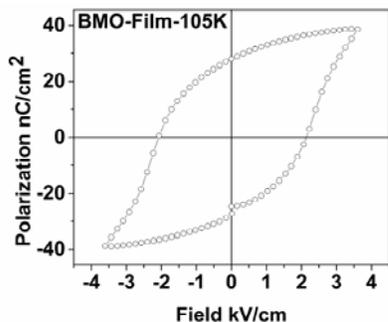
**Figure 3.** P-V hysteresis loop of a BMO thin film on a Pt/TiO<sub>2</sub>/SiO<sub>2</sub>/Si substrate at 105 K.
