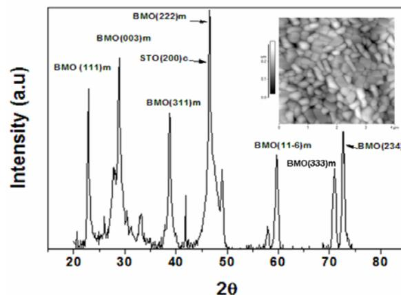
**Figure 1.** XRD and Atomic force microscopy (AFM) of a BiMnO<sub>3</sub> thin film on a SrTiO<sub>3</sub> (100) substrate. Inset shows the AFM image of a 100 nm thin film, note the grain size near 0.3 μm.
