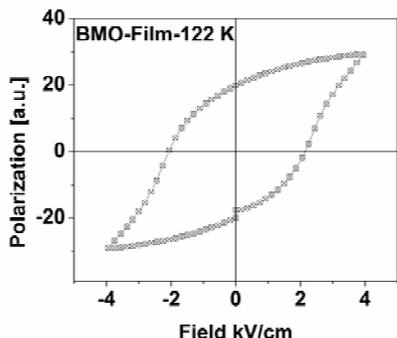
**Figure 4.** P-V hysteresis loop of a BMO thin film on a SrTiO<sub>3</sub> (100) substrate at 122 K.
