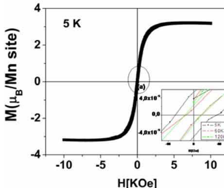
**Figure 6** Magnetic hysteresis loop for a BiMnO<sub>3</sub>/SrTiO<sub>3</sub>(100) thin film at 5 K. The zoom displays the region enclosed in the circle.
