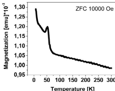
**Figure 7.** ZFC temperature dependence of the magnetization for a BiMnO<sub>3</sub>/SrTiO<sub>3</sub> (100) thin film in a field of 10000 Oe.
