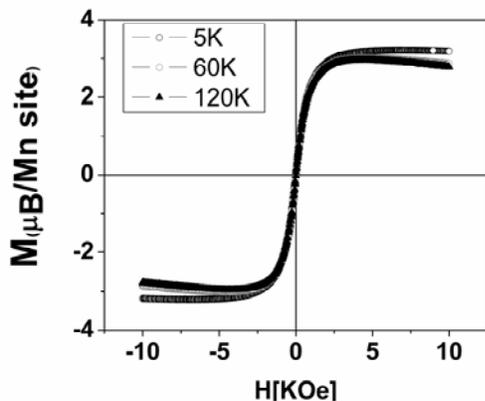
**Figure 5.** Magnetic hysteresis loops at different temperatures of BiMnO<sub>3</sub>/SrTiO<sub>3</sub>(100) thin films.
