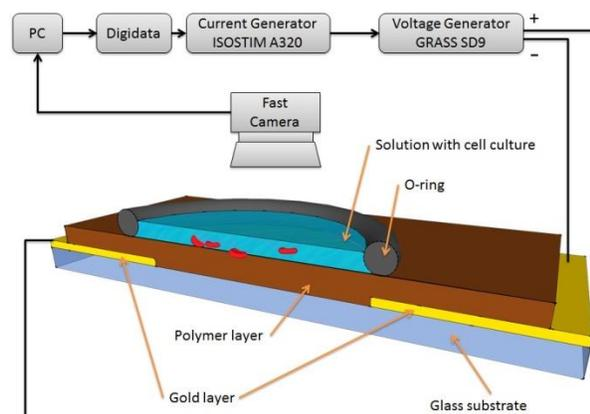
**Figure 2.** Experimental setup for excitation and measurement of the contractile response of the electrogenic cells (cardiomyocytes and muscle fibers). The excitation was delivered through the conducting polymer films only.
