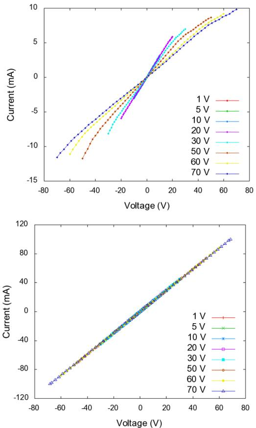
**Figure 4.** (a) Degradation of the conductance of the film made with PEDOT:PSS+SDS when the polarization voltage is highly increased. (b) Conductance stability for the film made with PEDOT:PSS+PEG and increasing polarization voltage.
