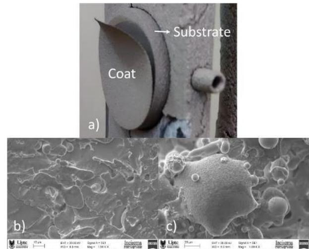
**Figure 8.** (a) Coating deposited according to the parameters of test No. 7. (b) The deposited splashes for test No. 8, which were in direct contact with the substrate (c) Splashes on the upper surface layer deposited according to the parameters for test No. 8.
