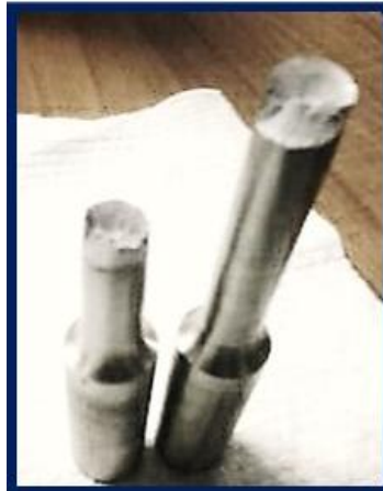
Figure 2. AA7075-T6 fractured specimens obtained at the end of the tensile test.
